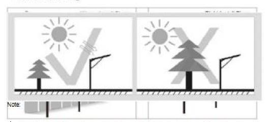
★ When install the integrated solar led street, please choose a posi-tion with enough sunshine and fully exposure. Pis note the solar panel must be fully exposured, without any shelter.
